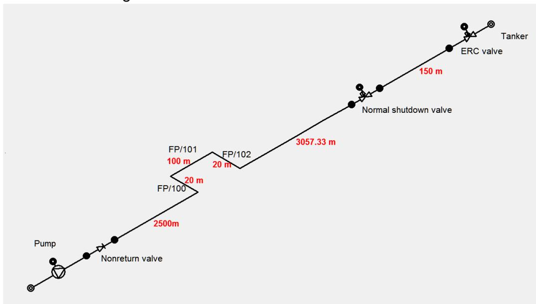
In the above schematic FP/100, FP/101 and FP/102 are the hydraulic transient forces which need to be calculated.
